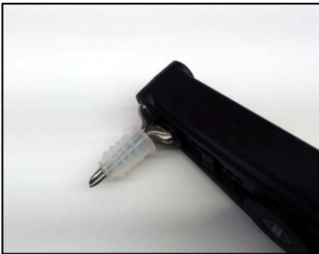
FIGURE 8 - PROTECTIVE SHROUD PLACED ON TOOL
